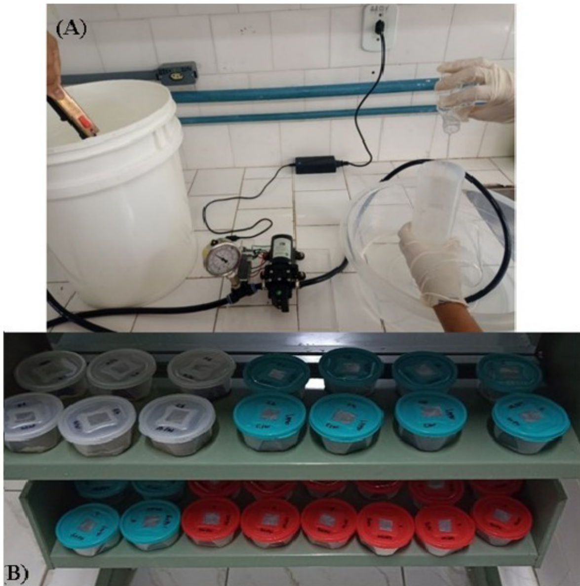
Figure 1. (A) Passage of entomopathogenic nematodes through the pressure system. (B) Biological assay to evaluate the mortality of Stomoxys calcitrans larvae caused by entomopathogenic nematodes.
